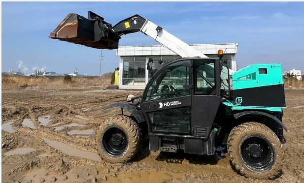
Demo of Telehandler to which Full Hybrid Powertrain is Applied
