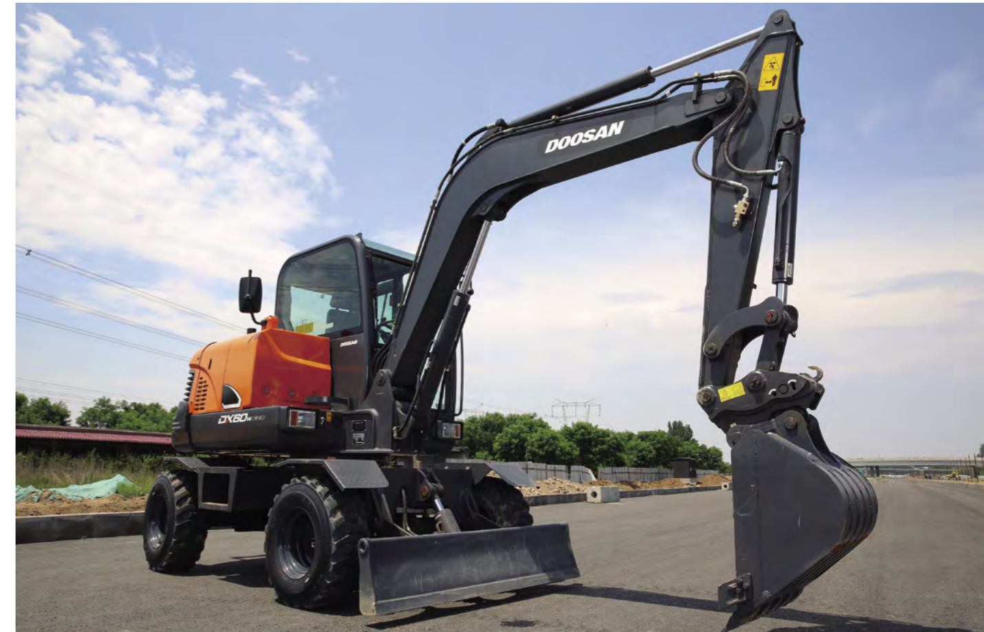
DX60W ECO, a 6-ton low-end wheel excavator launched for the Chinese market in 2020
